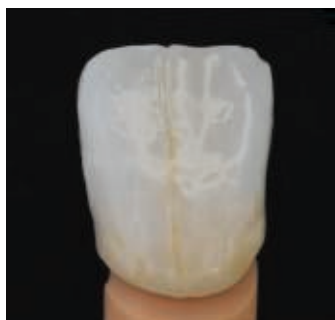
KATANA™ Zirconia STML NW FC Paste Stains - Cervical 2, B+, White, Grayish Blue, Clear Glaze
