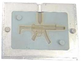
The tested polymers are listed in the table below and include PP, PE, HDPE, ABS, PETG, PA6 and PA12 co-polymer, injected at temperatures between 230 and 280°C (446 - 536°F). All materials were injected without any mold release agents.
