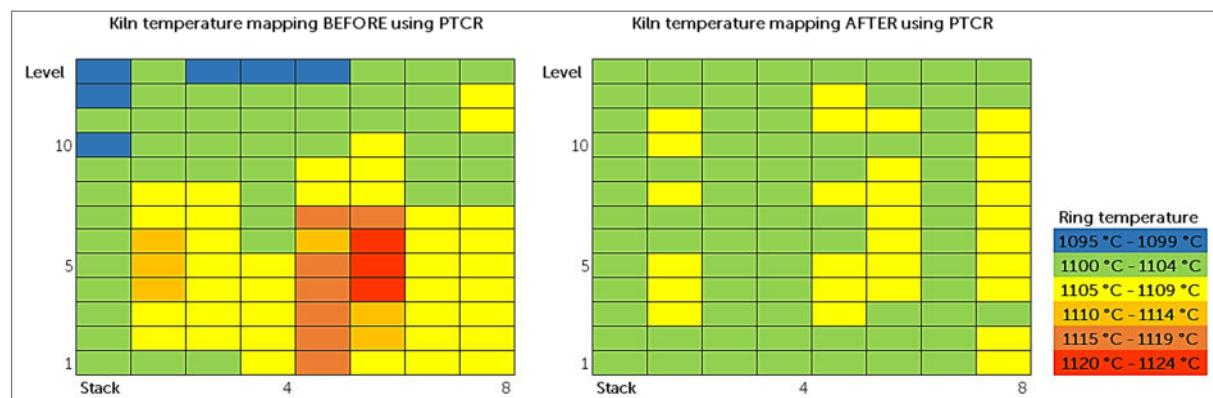
The most frequent use of PTCR is by optimising and managing the firing/sintering processes to achieve the optimal product quality and to assess the thermal performance and characteristics of a kiln/furnace. The way of working is to make a number of runs with different settings of the parameters temperature and time. These runs are characterised by the ring temperature (RT) values as determined from the rings. Product quality analysis determines the optimal run and accompanying RT values.
